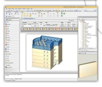
**SAPFIR-Structures** module enables you to generate design model of the structure based on 3D model obtained in SAPFIR-3D, Allplan, Revit, AutoCAD, etc.
