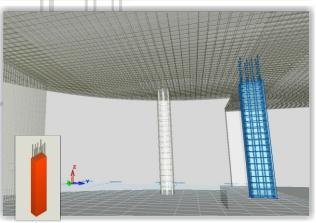
According to mosaic plots of design reinforcement on the model of whole structure, in COLUMN module you could obtain tools to generate required types of reinforcement for defined marks of columns. Column reinforcement is arranged automatically according to assigned type of reinforcement. Rebar pattern generated automatically may be modified by the user later.
